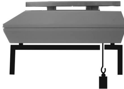
Fig. 1: Setup of balance for underfloor weighing
